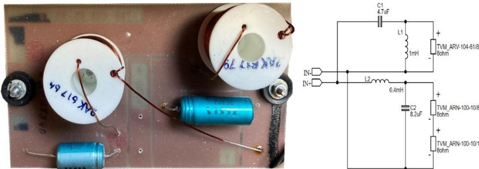
Fig. 7.28 Crossover used in multifunction speaker with scheme
