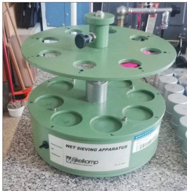
Figure 10. Wet Sieving Apparatus (Eijkelkamp). Author of the photo: Marley Whanda Figueroa Jiménez.
