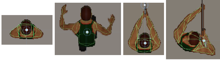
Figure 7.6: Hitboxes (green lines) from left to right: Standing Idle, Crouching Idle, Short Weapon Equipped and Long Weapon Equipped.
