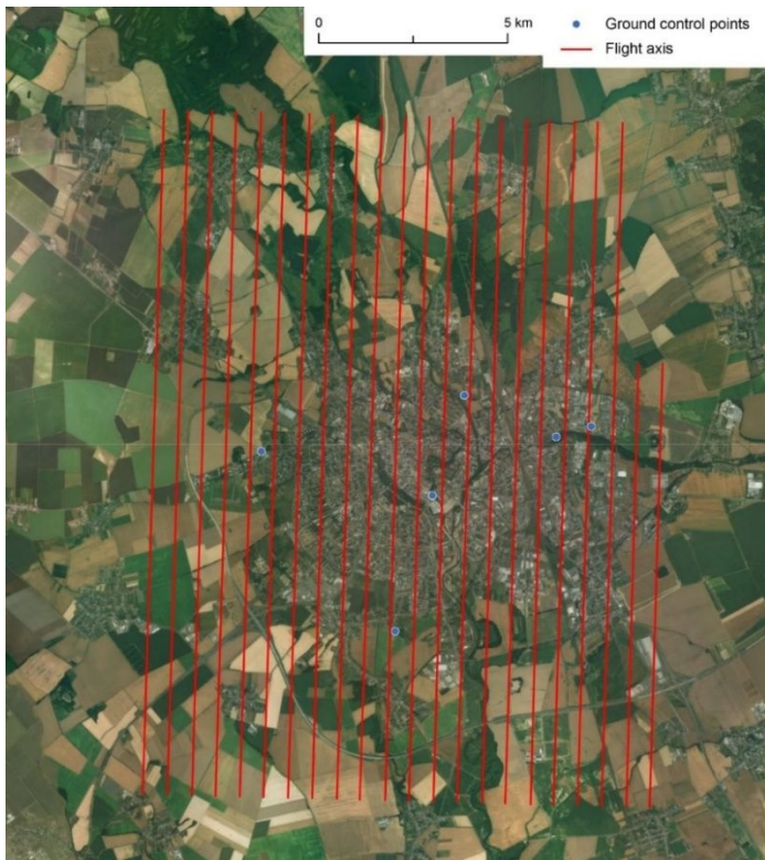
Figure 2 Flight lines and ground control locations over the Olomouc city. The flight was carried out from the west towards the east. In red, the planned flight lines are visualised. Blue dots symbolise the ground truth data locations.
