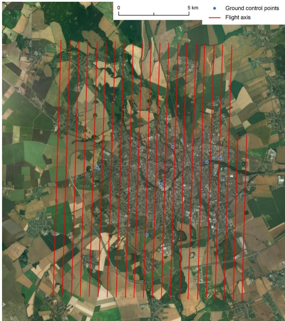
Figure 5.1 Flight lines and ground control locations over the Olomouc city. The flight was carried out from the west towards the east. In red, the planned flight lines are visualised. Blue dots symbolise the ground truth data locations.
