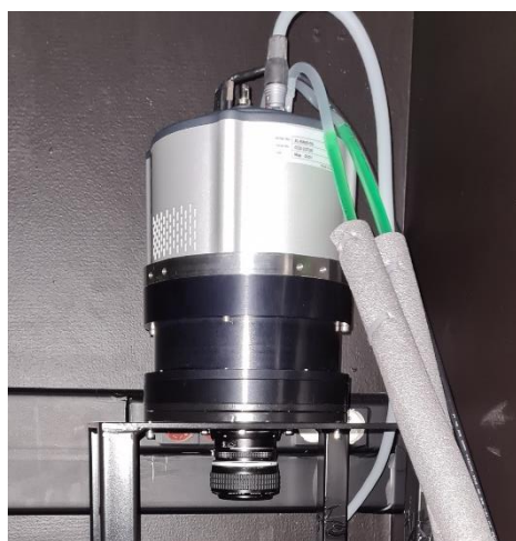
Figure 4. The new CCD camera, with visible water-cooling pipes and attached objective and a stand construction.
