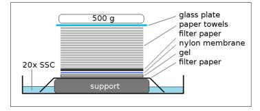
Fig. 2. 5 Layout of arrangement used for capillary transfer of DNA from agarose gel to a nylon membrane.
