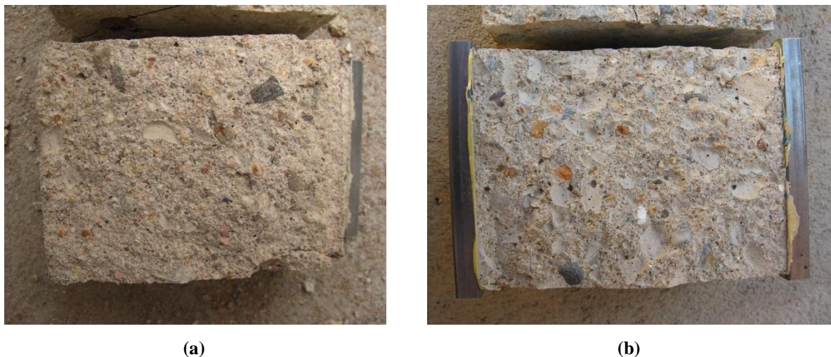
Figure 8-18 : Fracture plane – (a) Specimen R3K_II_1C, (b) Specimen R5I_2C
