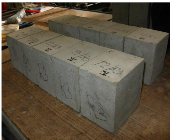
Figure 5-7 : Sawed standard beam-shaped testing specimen
