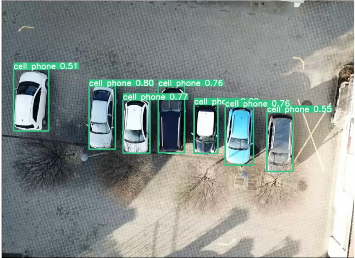
Figure 6.6: Cars are detected incorrectly as cell phones when the source image is taken from a top-down view.
