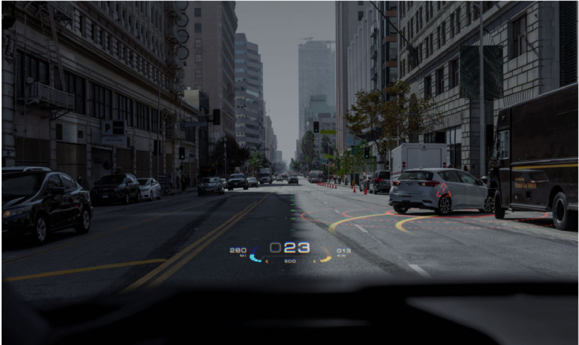
Figure 2.1: AR Heads Up Display integrated into a car windshield. 1
