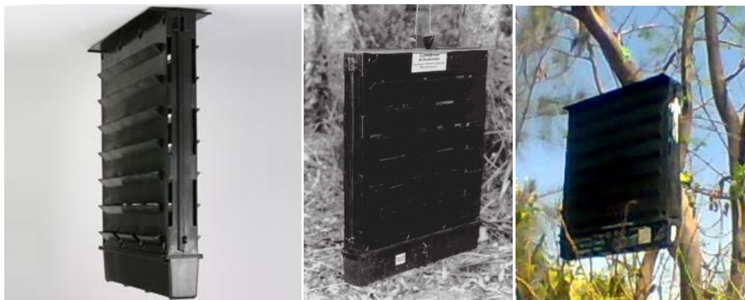
Fig. 2. Theysohn pheromone slot traps (Ridex s.r.o., Vrbno pod Pradědem, Czech Republic), hanged on trees in experimental area.
