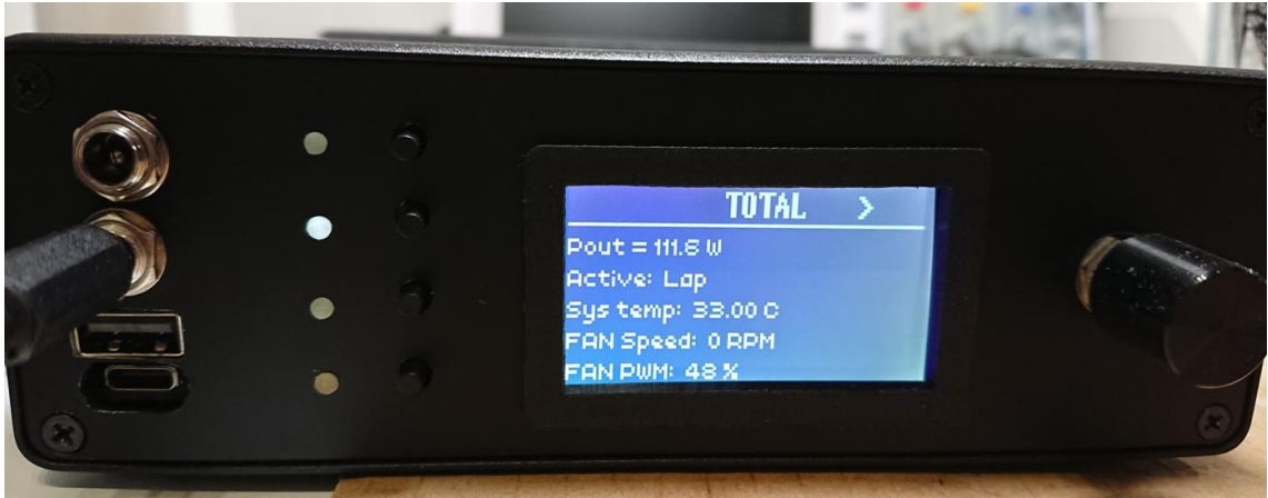
Fig. 6.3 The test of maximum output power
