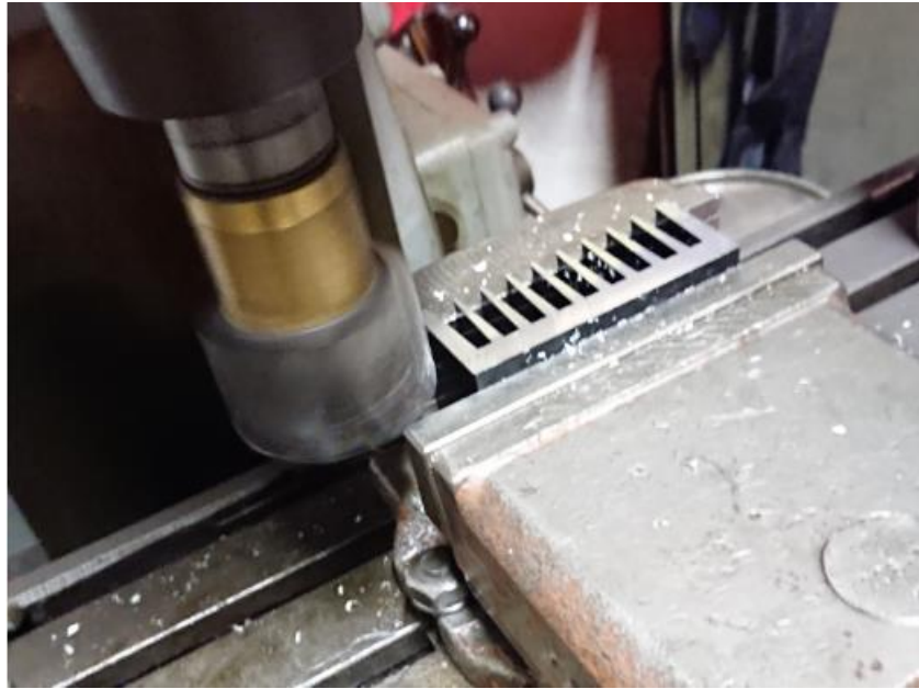
Fig. 4.17 Milling of the heatsink
