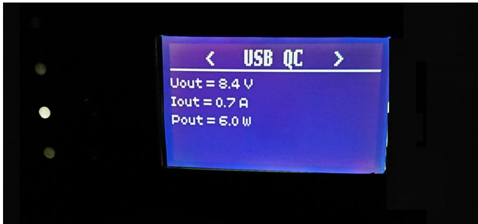
Fig. 6.1 Smartphone charging via the USB-A Quick Charge output
