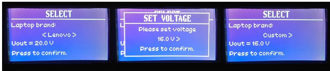
Fig. 5.4 Setting the laptop output voltage
