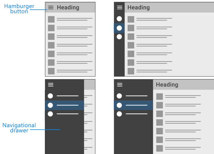
Figure 2.2: Navigational Drawer and its appearance on small and large displays.
