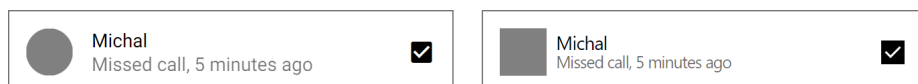
Figure 4.7: Example of an item with an avatar, two lines of text and a checkbox, created using [fx-item] attribute. Material Design variation is on the left, Neon design on the right.
