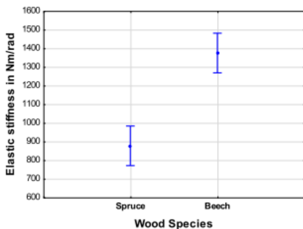
Fig. 6. The effect of wood species on elastic stiffness.
