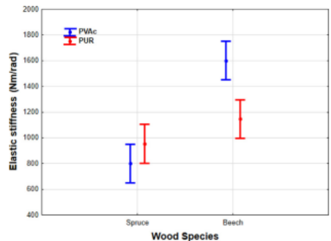
Fig. 7. The effect of adhesive type on spruce and beech wood elastic stiffness.
