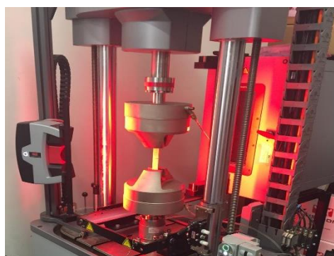
Figure 7 Shear test sample attached to the UTM (Universal testing machine) with video extensometer
