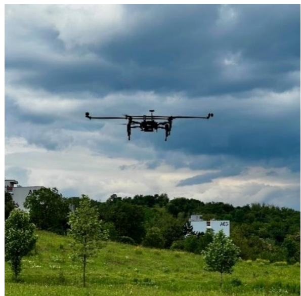
Figure 45: the DJI M100 UAS fitted with two Calypso anemometers during the initial flight tests.
