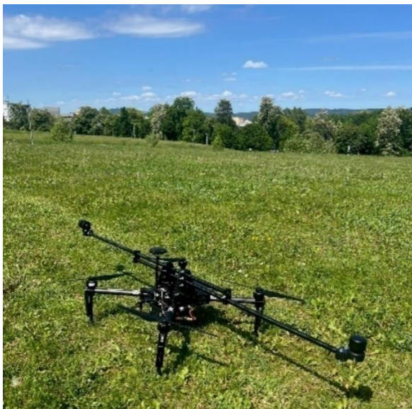
Figure 45: the DJI M100 UAS fitted with two Calypso anemometers during the initial flight tests.
