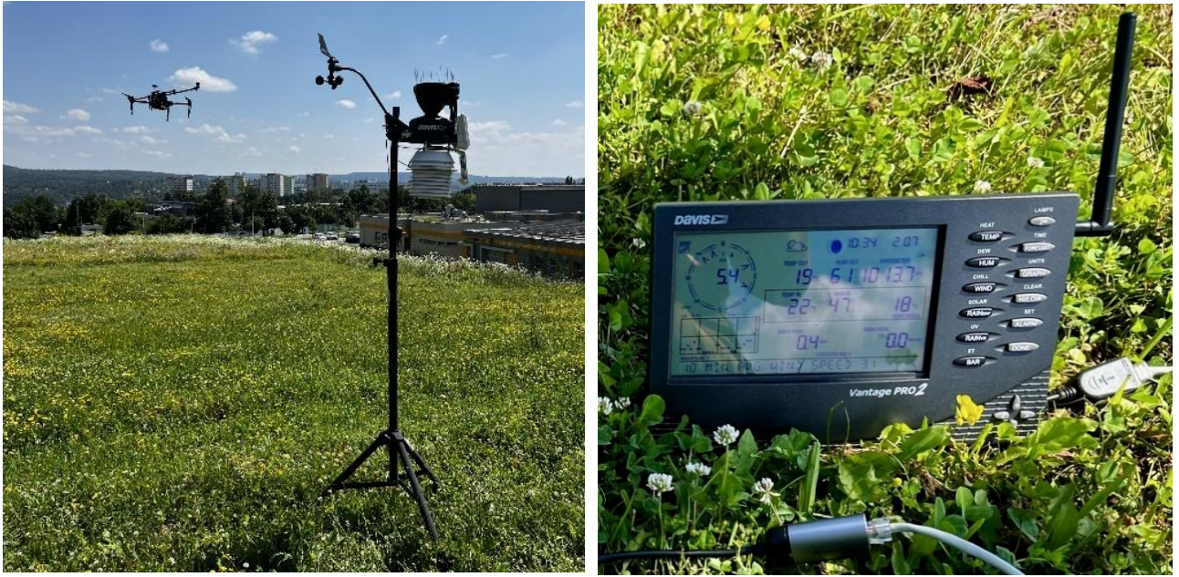
Figure 46: ground-based reference, meteorological station Davis Vantage Pro2 during UAS test flight.
