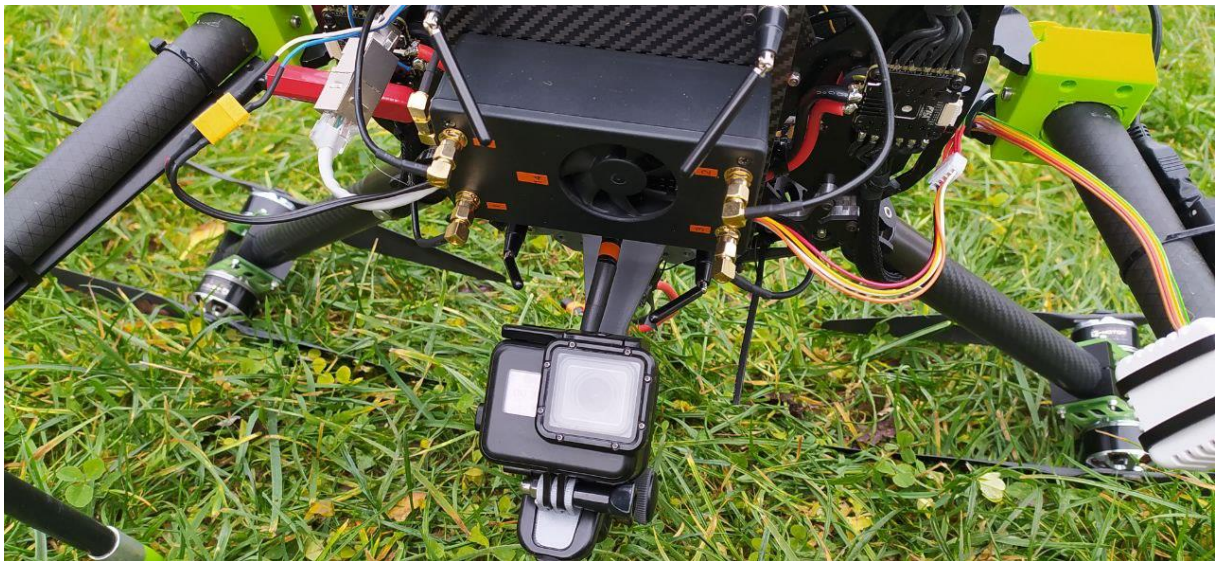
Figure 3: Honeywell SC-Modem (black box with fan) and sensors case included two meteorological sensors (white box on drone leg).
