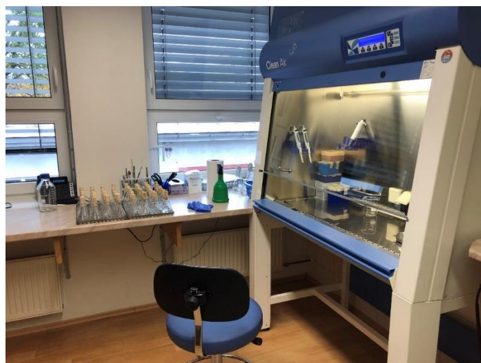
Figure S2. Sterile flow-box used for the inoculation of picocyanobacteria cultures (author's photo)
