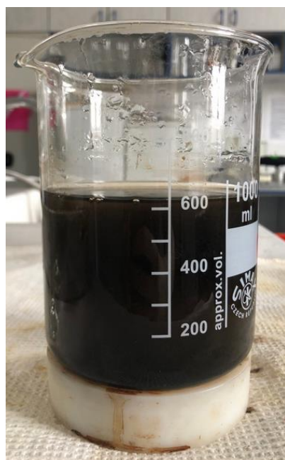
Figure 18. Microwave synthesized magnetite on the NdFeB magnet (author's photo)
