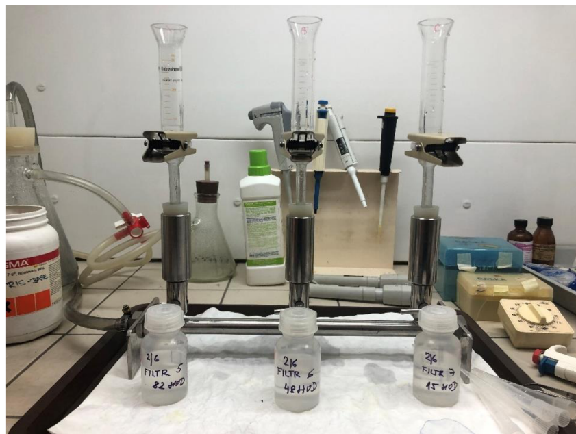
Figure 14. The apparatus used for the purpose of DAPI staining of picocyanobacterial cells and counting filter preparation (author's photo)
