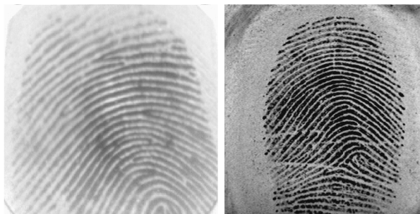
Figure 4.2: Two fingerprint images acquired by optical scanners with different sensing areas. On the left, a scanner with an insufficiently small sensing area was used. Images obtained from FVC 2000 [28].
