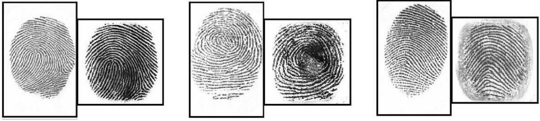
Figure 7.4: Fingerprint examples from MCYT Fingerprint subcorpus [31]. Fingerprint images are given for the same finger for both capacitive acquisition (left in each panel) and optical acquisition (right in each panel), and three different fingerprints in the database, one per column.
