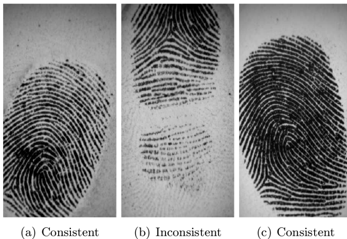
Figure 4.4: An example of three fingerprint images of the same finger with different consistency. Wrong finger placement on the sensor plate caused the inconsistent fingerprint sample (b). Images were obtained from FVC2002 [26].
