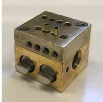
Figure 20: A holder is able to grip up to 8 copper tubes in order to freeze-fracture and image the sample inside.
