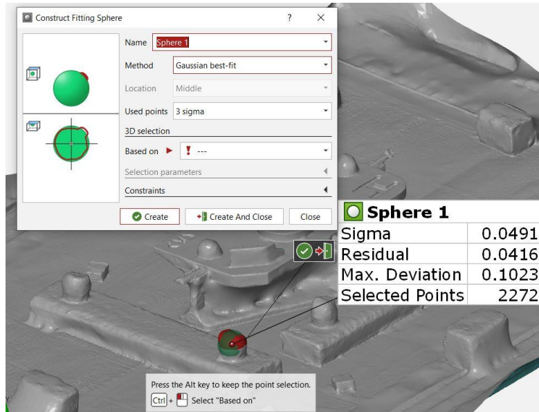
Figure 30: Creation of spheres using Gaussian best fit method
