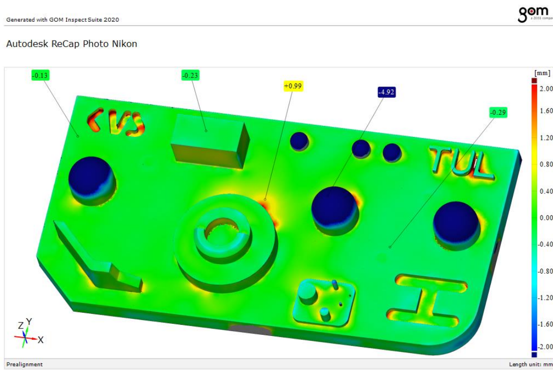
Figure 47: Colour map of deviations of Autodesk ReCap Photo from Nikon Camera
