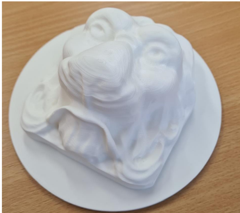
Figure 8: 3D printed model from ATOS Triple Scan
