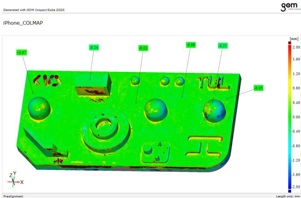
Figure 51: Colour map of deviations of COLMAP Software from iPhone camera
