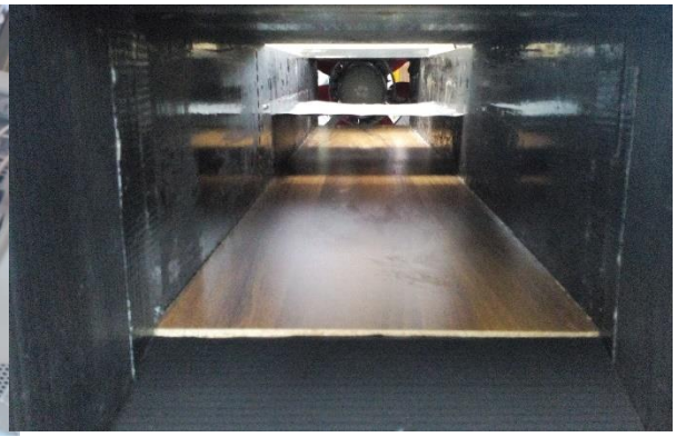
Figure 23 Sheets placed inside the test section at mid height of the wall
