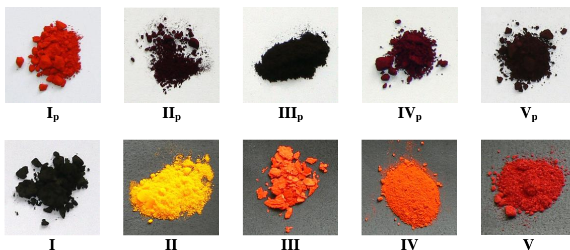
Figure 35: Polycrystalline photos of DPP I to V made under daylight with a Panasonic DMC-FZ7 camera.
