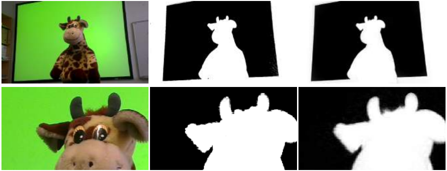
Figure 6.4: left: The original image from the camera. middle: Matting results from GPU shaders. right: Reference alpha mask acquired using KNNmatting with manual annotation.
