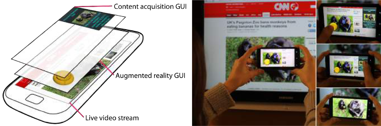
Figure 5.4: Left: GUI layers of the content requester application. Right: The migration process.
