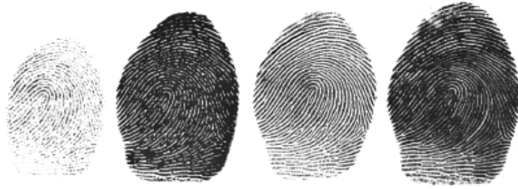
Figure 2.5: Fingerprint samples acquired from the same finger with skin subjectively perceived as (left to right): dry (62.5 %), wet (99.9 %), normally moist (84.6 %), and normally moist (84.6 %) with finger strongly pressed against the sensor [32].
