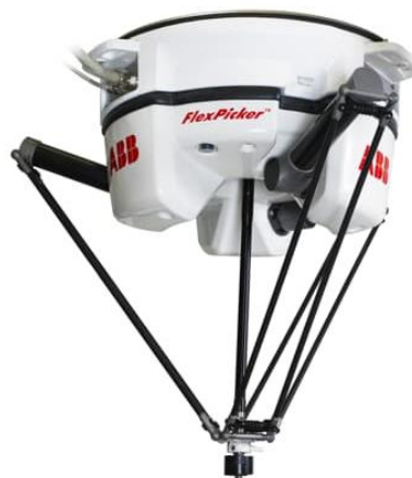
Obr. 5) Delta robot ABB IRB 360 Flex Picker [11]
