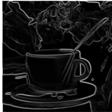
Figure 3: original Canny/Deriche filter applied. Alpha parameter set to 3.8 to produce similar output as the edge detector below
