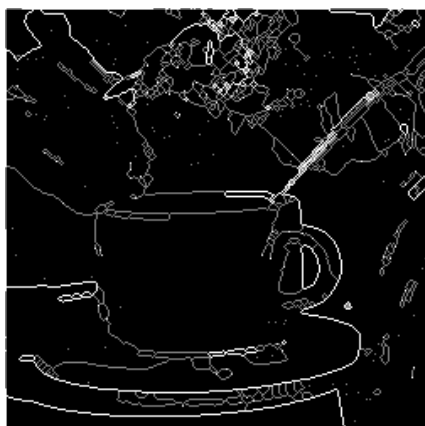
Figure 16: thinning applied (after edge detection)
