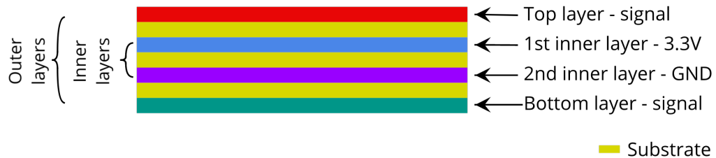
Fig. 2.19: The 4-layer PCB stackup.
