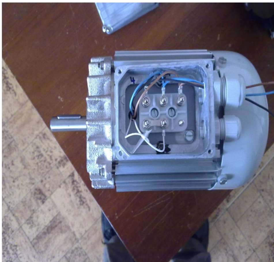
Figure 12: Induction motor connected in star and delta.
