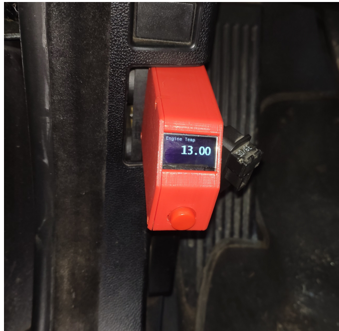
Fig. 7.3: OBDII diagnostic tool – testing in BMW E91.
