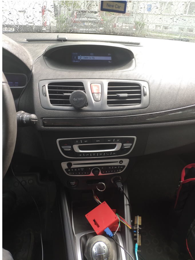
Fig. 7.4: OBD II monitoring device – testing in Renault Megane.
