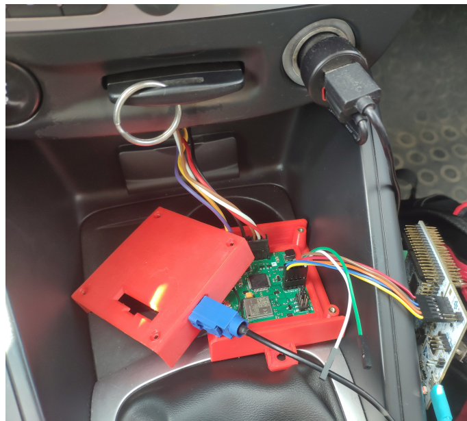
Fig. 7.5: OBD II monitoring device – testing in Renault Megane – closeup.
