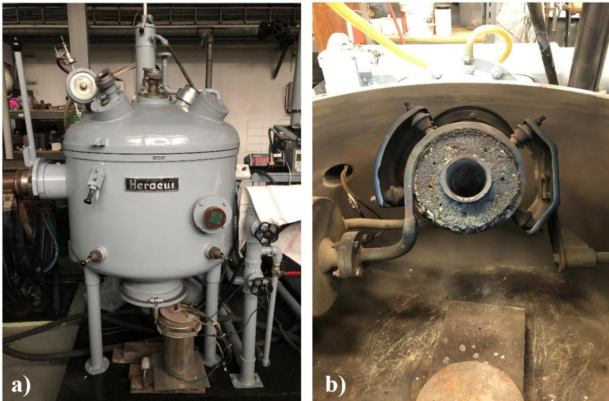
**Fig. 9** Heraeus vacuum induction equipment in VUT FSI for melting, processing, and casting in vacuum or an inert atmosphere (max. Approx 20k) (a) vacuum induction furnace IS2/ I HERAEUS; (b) zirconia ZC93i crucible for metal handling and melting.
