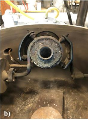
Fig. 9 Heraeus vacuum induction equipment in VUT FSI for melting, processing, and casting in vacuum or an inert atmosphere (max. Approx 20k) (a) vacuum induction furnace IS2/ I HERAEUS; (b) zirconia ZC93i crucible for metal handling and melting.
