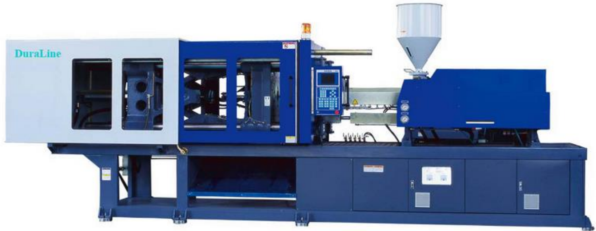
Figure 5-1-2. An example of a Plastic injection moulding machine. DuraLine Group, United States, Model: 1075 Clamping forces: 600 to 60,000 kN.
