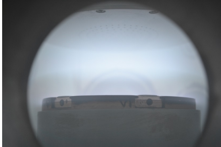
Fig. 17: Photo of electrodes during deposition (below rotational electrode with sample holders)
