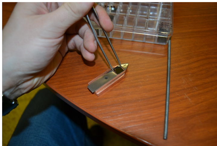
Fig. 15: Loading silicon wafer sample to sample holder
