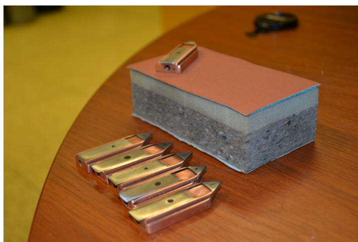
Fig. 28: Cleaning sample holders by sandpaper
