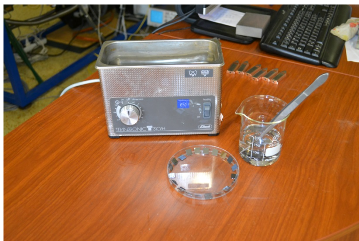
Fig. 27: Cleaning samples by ultrasonic bath and preparation of samples to drying
