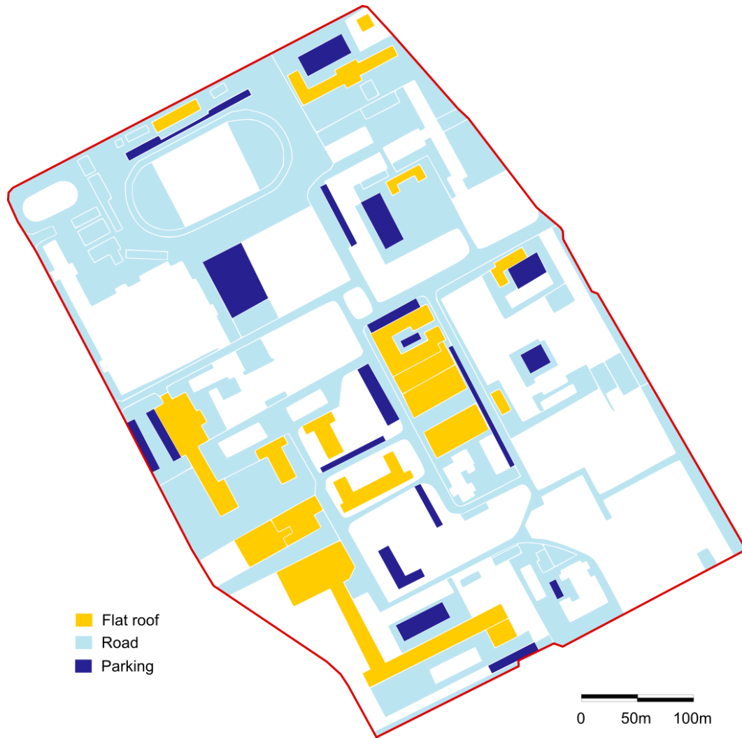
Figure 21: Layout of retrofit areas – all flat roofs to green roofs and all pavements (parking lots and roads) to semi-green surfaces. Blank area presents the non-modified surfaces as existing green area and all sloped roofs.
