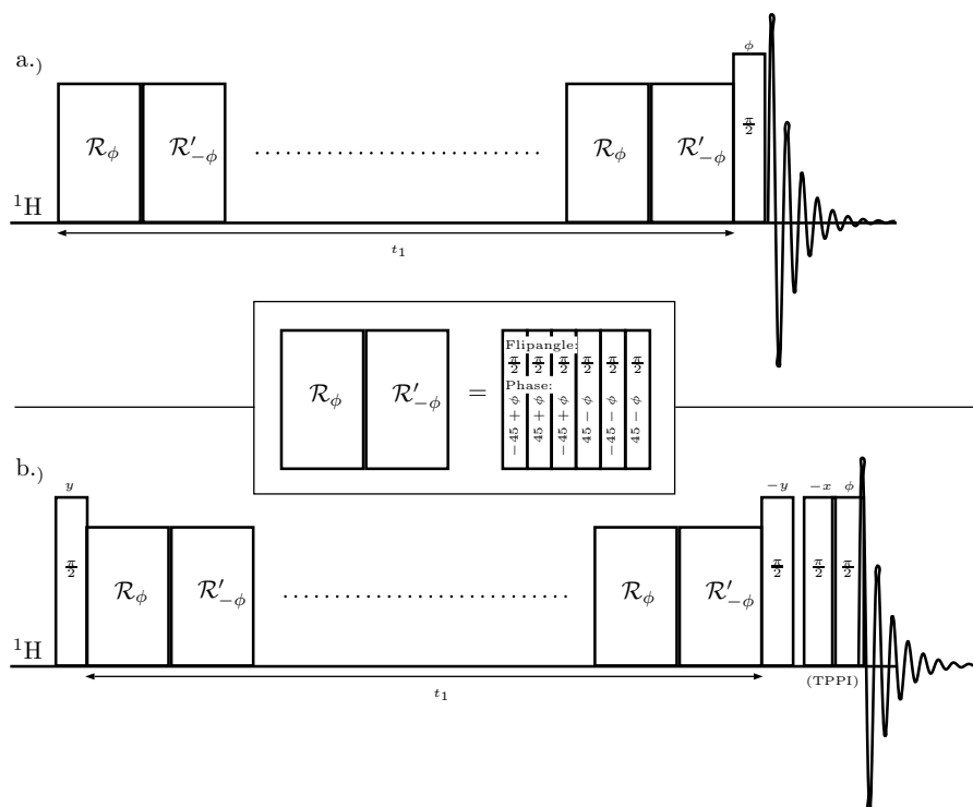
Figure 1.35.: Pulse sequence schemes for experiments giving high resolution ^1\text{H} spectra. One \mathcal{R} block consists of three \frac{\pi}{2} pulses with different phases, which form a composite \pi pulse (box in the middle). [2] a.) shows a basic version of the sequence with t_1 incremented \mathcal{R} decoupling followed by a phase cycled detection pulse. [2] b.) gives an enhanced version with two \frac{\pi}{2} pulses flanking the decoupling block, an additional pulse before acquisition and TPPI. [3]
