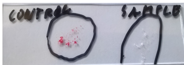
Figure 4.7.: Comparison of the outcomes of the test for free -OH groups with unloaded Wang resin (labelled with ' CONTROL ') and Fmoc-Phe loaded Wang resin (labelled with ' SAMPLE ')
