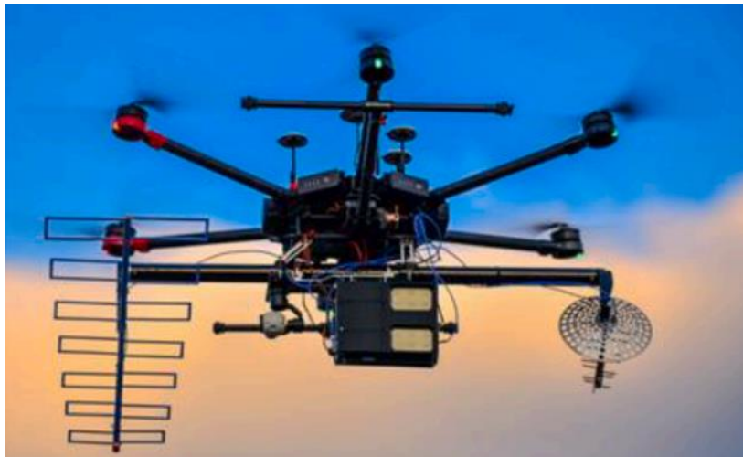
Figure 8. An example of UAV-SAR equipped with P-, C-, and L-band antennas (Asadzadeh et al., 2017).
