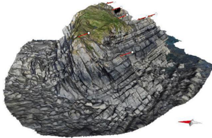
Figure 4. A detailed virtual outcrop constructed by mosaicking close-up images (Cawood et al., 2017).
