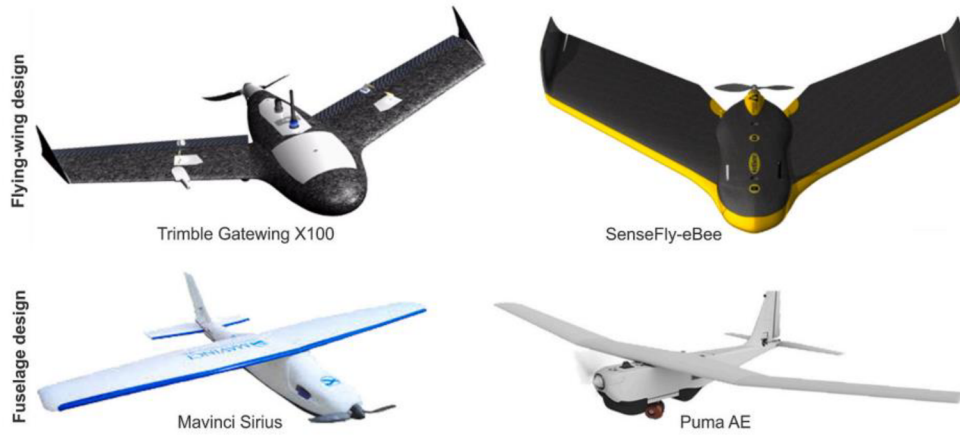
Figure 5. Examples of lightweight fix-wing commercial drones ( Asadzadeh et al., 2017).
