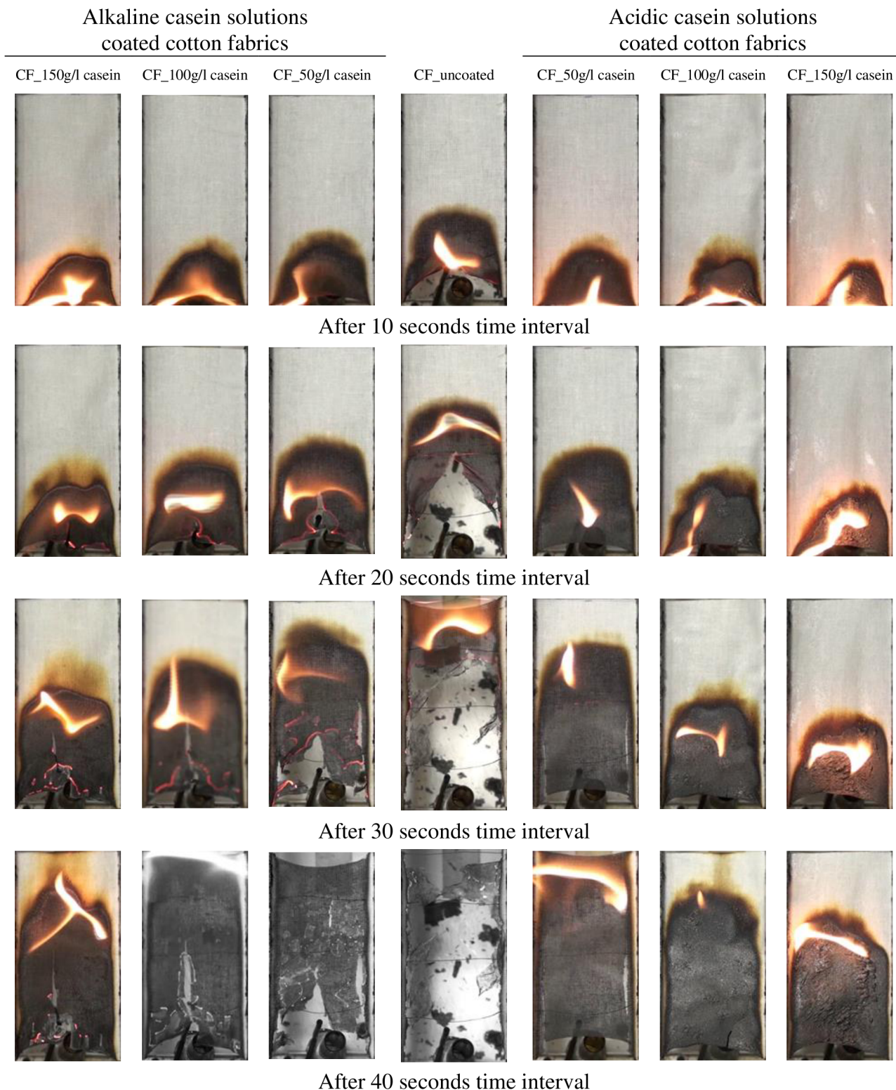
Figure 5.14. Photographs of burnt uncoated and casein coated cotton fabrics at different time intervals during flame test
