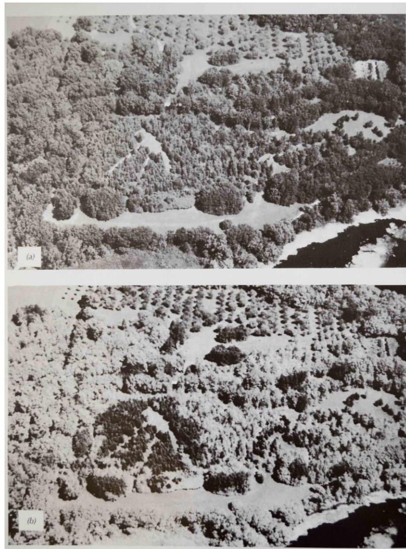
Figure 25: Low altitude oblique aerial photographs illustrating deciduous versus coniferous trees. (a) Panchromatic photographic recording reflected sunlight over the wavelength band 0.4 to 0.7 \mu\text{m} . (b) Black and White infrared photograph recording reflected over 0.7 to 0.9 \mu\text{m} wavelength band (Lillesand et al., 2000).
