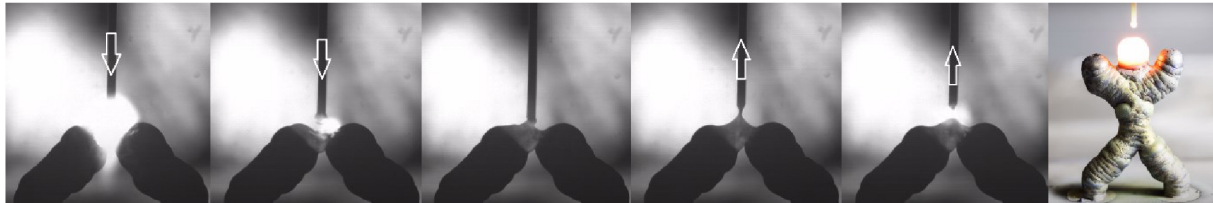
Obr. 34: Proces CMT Cycle Step [32]
