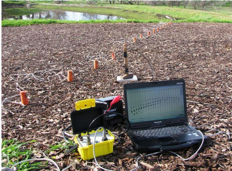
Figure 18 Set-up of geophones. Depicted is also a central unit (geostuff.com, n.d.).
