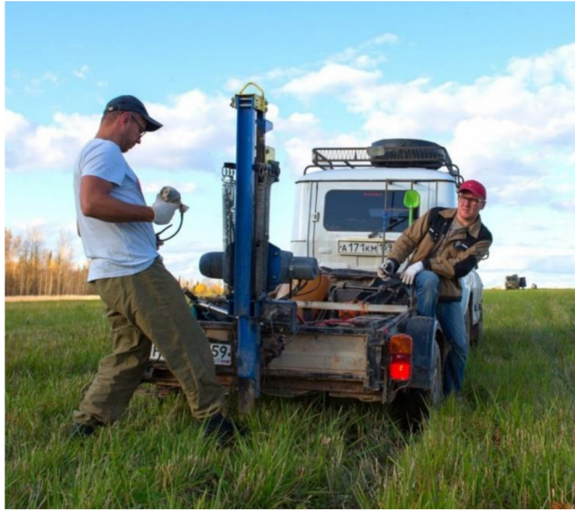
Figure 14 Mechanical hummer that generate vibration in seismic survey (Geodevice, n.d.).
