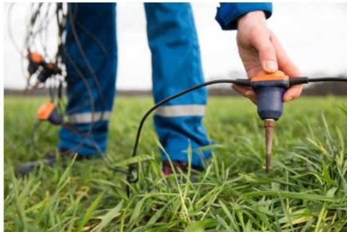
Figure 17 Land geophones that are utilized in the land seismic survey (geostuff.com, n.d.).
