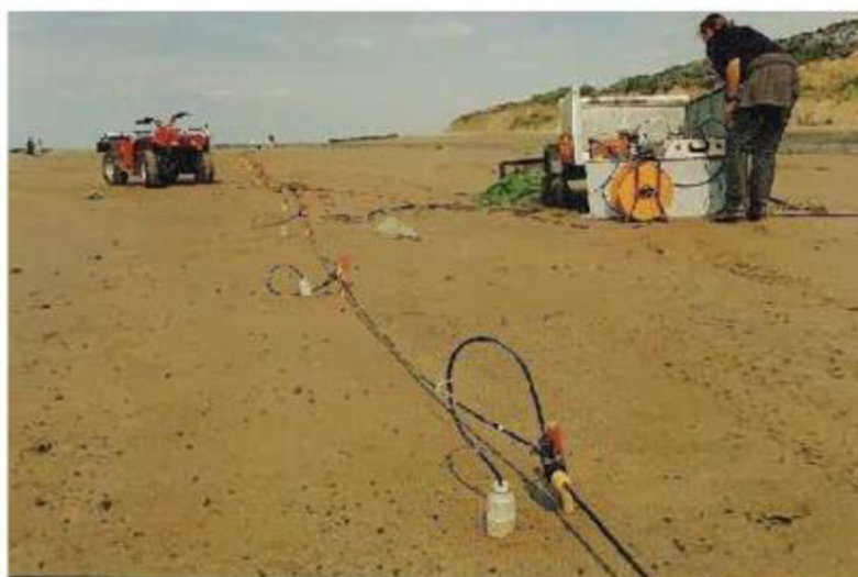
Figure 4 Array of geophones connected by a cable during a shallow seismic data gathering (volcano n.d.).
