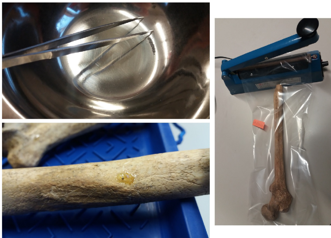
Figure 9.9: Marking the bone fragments with tantalum ( left ) beads and packing into the foil sleeve ( right ).
