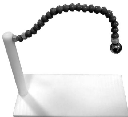
Figure 3.1: Lombardi self-holding X-ray magnification marker. Retrieved from Innomed, Inc. 1 .
