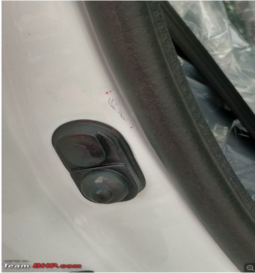
Figure 26 Found Paint chipping in the rear passenger door during PDI
