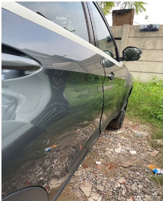
Figure 25 Gap found on the driver side door of new Tata Nexon. Source: medium.com
