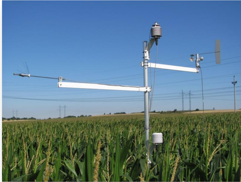
Photo 8.4.1: Bowen-ratio sensor installed in corn field (©Pivec, 2013).
