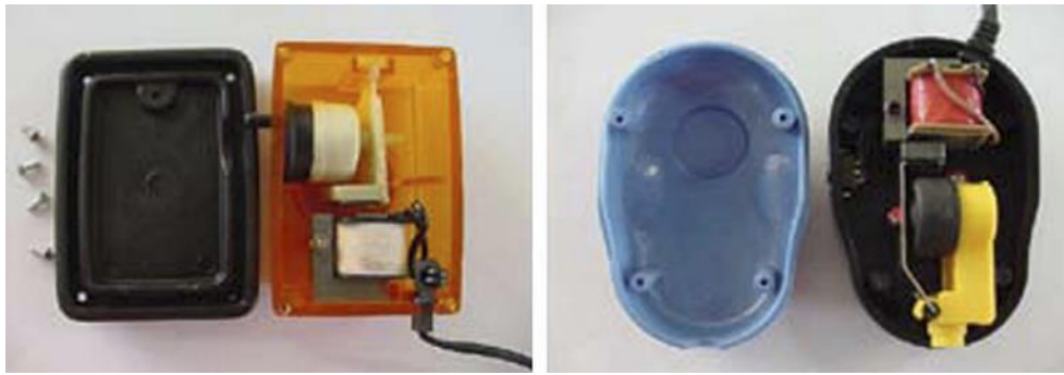
Fig. 2-10 Internal design of compressors for aquariums [9].
