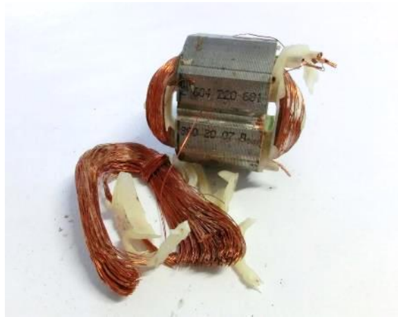
Fig. 5-7 Photography of stator with removed one winding.
