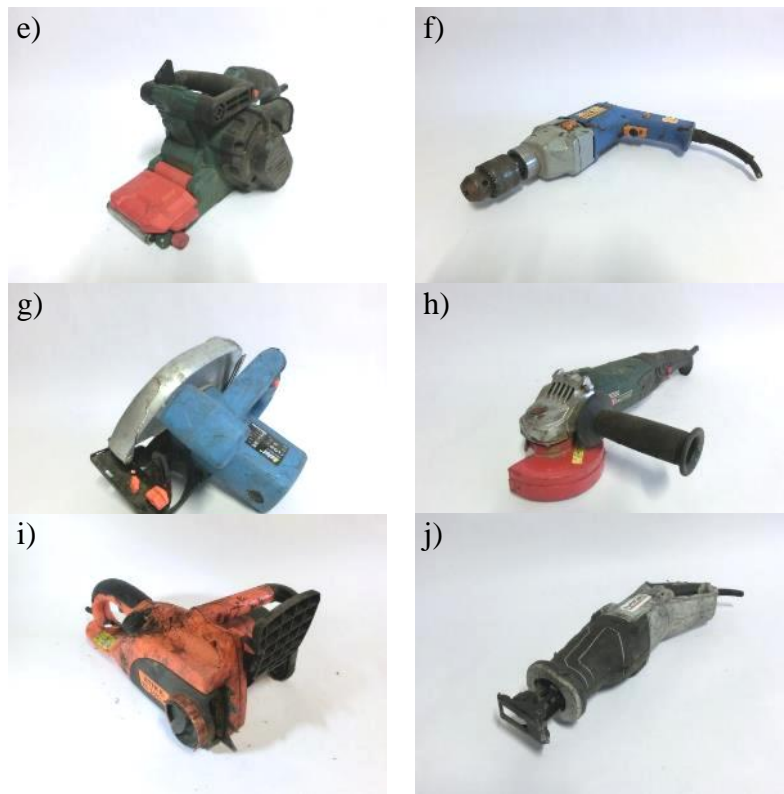
Fig. 6-9 Example of power tools; (a) Random Orbital Sander – OS5; (b) Sheet Sander – (SS8); (c) Electric Planer – (EP3); (d) Handle Jigsaw – HJ11; (e) Belt Sander – BS7; (f) Percussion Drill – PD2; (g) Circular Saw – CS7; (h) Angle Grinder – AG19; (i) Electric Chainsaw – EC13; (j) Reciprocating Saw – RS6.
