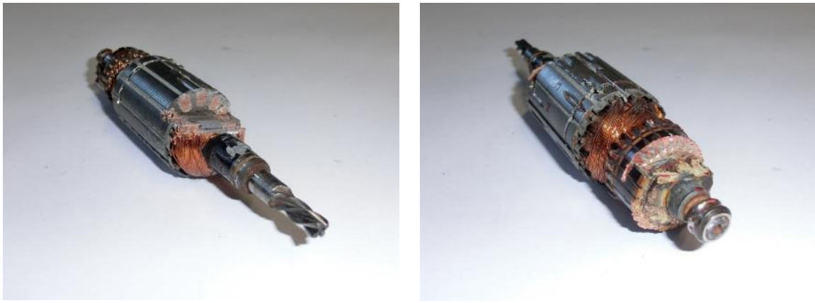
Fig. 5-8 Photography of rotor; (left) cut of armature; (right) cut of cummutator.
