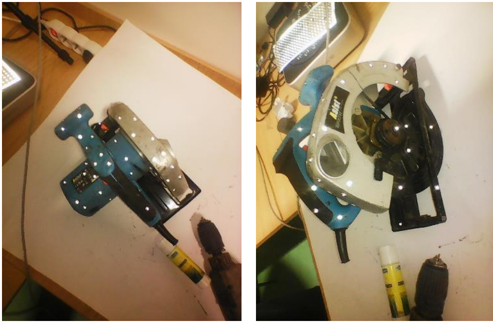
Fig. 5-5 Applied marking points for Circular Saw – Asist AE5KR120N; (left) marking points; (right) marking points.
