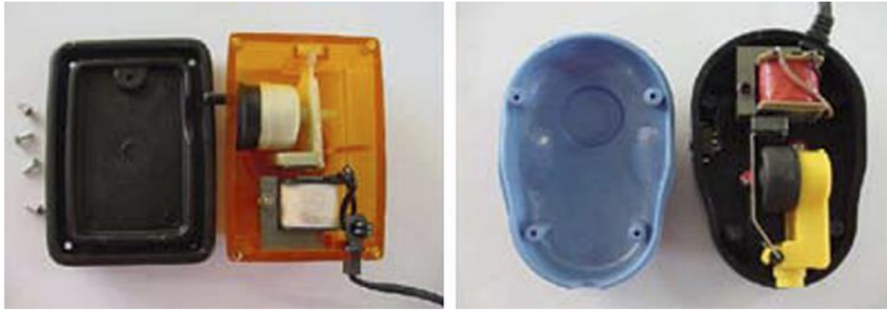
Fig. 2-10 Internal design of compressors for aquariums [9].
