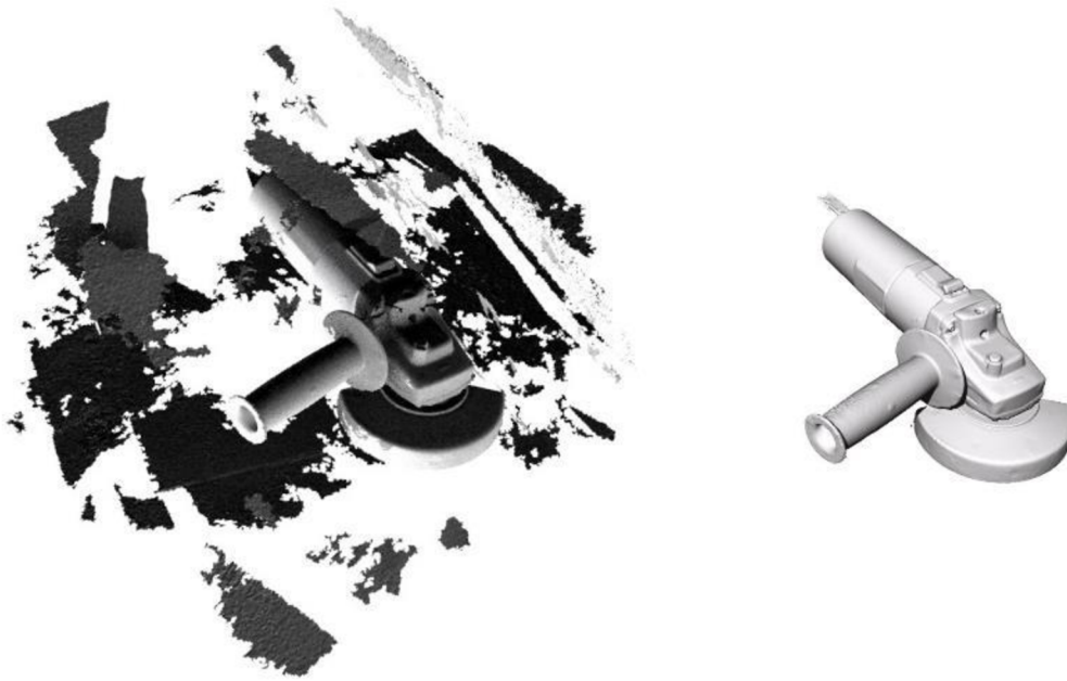
Fig. 5-6 Rhinoceros 7, imported STL Angle Grinder – narex EBU 13; (left) imported model; (right) cleared model.
