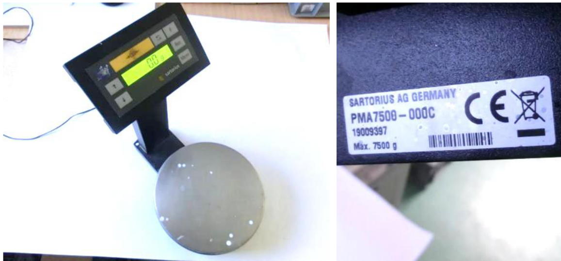
Fig. 5-1 Scale SARTORIUS PMA7500 – 00; (left) view of device; (right) product label.
