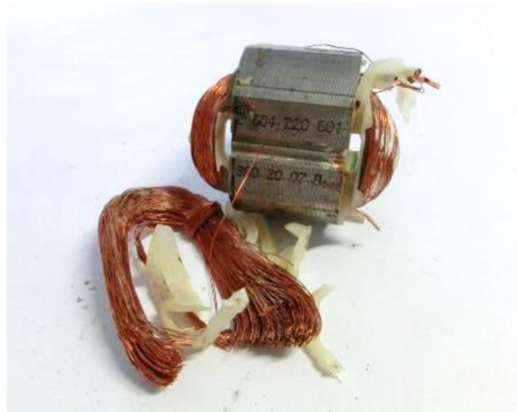
Fig. 5-7 Photography of stator with removed one winding.
