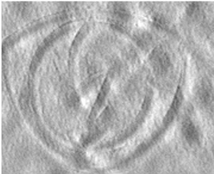
Figure 2.4. AFM vector lithography on the piece of compact disc (scan area is 6 \times 6 \mu\text{m}^2 )
