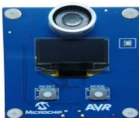
Obrázek 2.15: Core Independent Ultrasonic Distance Measurement with ATtiny817 - AVR42779 [16].
